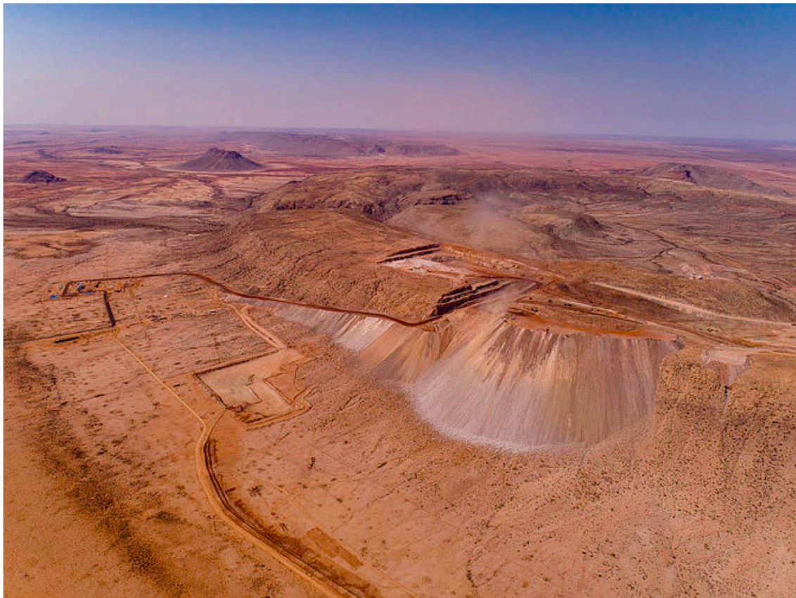
Figure 4a. Aerial view of Gamsberg in mid-2017, showing recently completed access ramp, v-cut and the beginnings of a very large ‘waste rock pile’. The plateau behind will eventually all be mined to depth, as shown in Fig. 4b.
